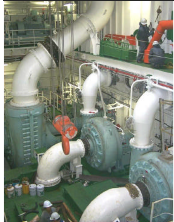
Hopper ship equipped with GIW double wall pump and two LSA jet water pumps.
